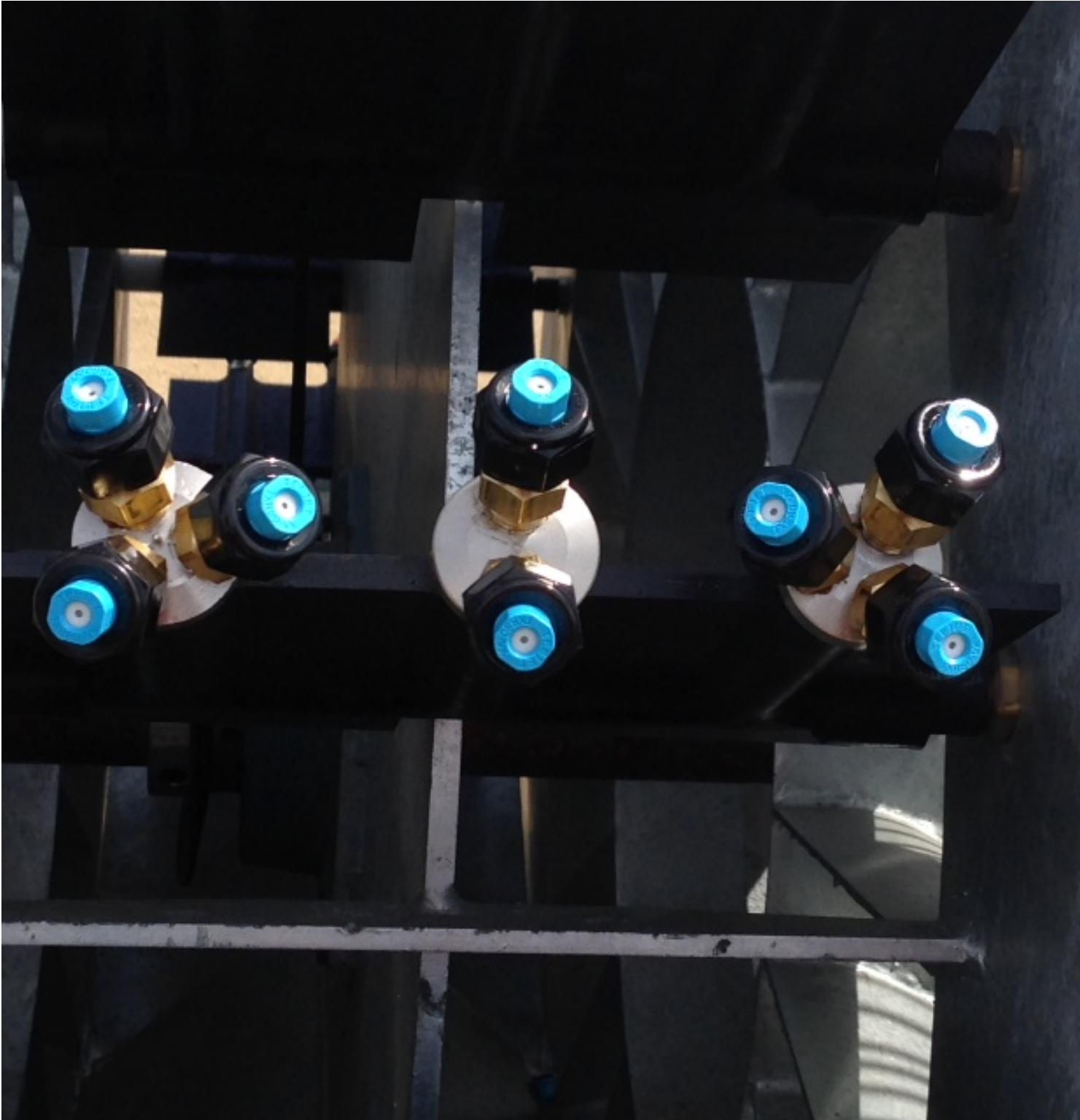
Figure 1. The new TXR Spray Systems nozzle configuration. Photo by Dr. Joel Siegel.
